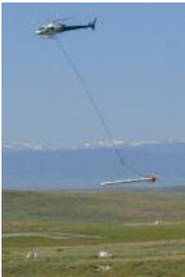
DOE is using remote sensors suspended from helicopters to map the flow of groundwater.
